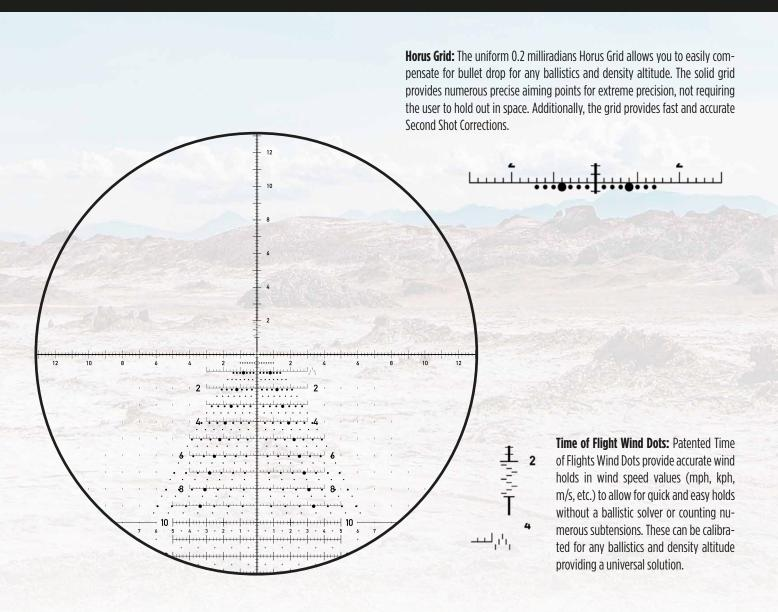
**Highly-Refined Mil Markers:** Refined "Chevron" mil markers throughout the reticle subtend to 0.1 milliradians to provide precise target range estimation. Vertical Chevrons are ideal for milling target height and the horizontal Chevrons for milling target width.
